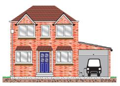
Where parking, other than a covered car park, is provided within the curtilage of a dwelling, a minimum of one electric vehicle charge point socket with an output rating of not less than 7 kW should be provided adjacent to the parking space.
